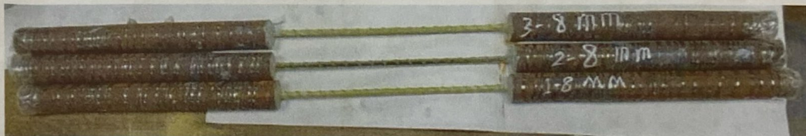
Fig. 1: Tested Samples with Installed Anchors Before Testing
